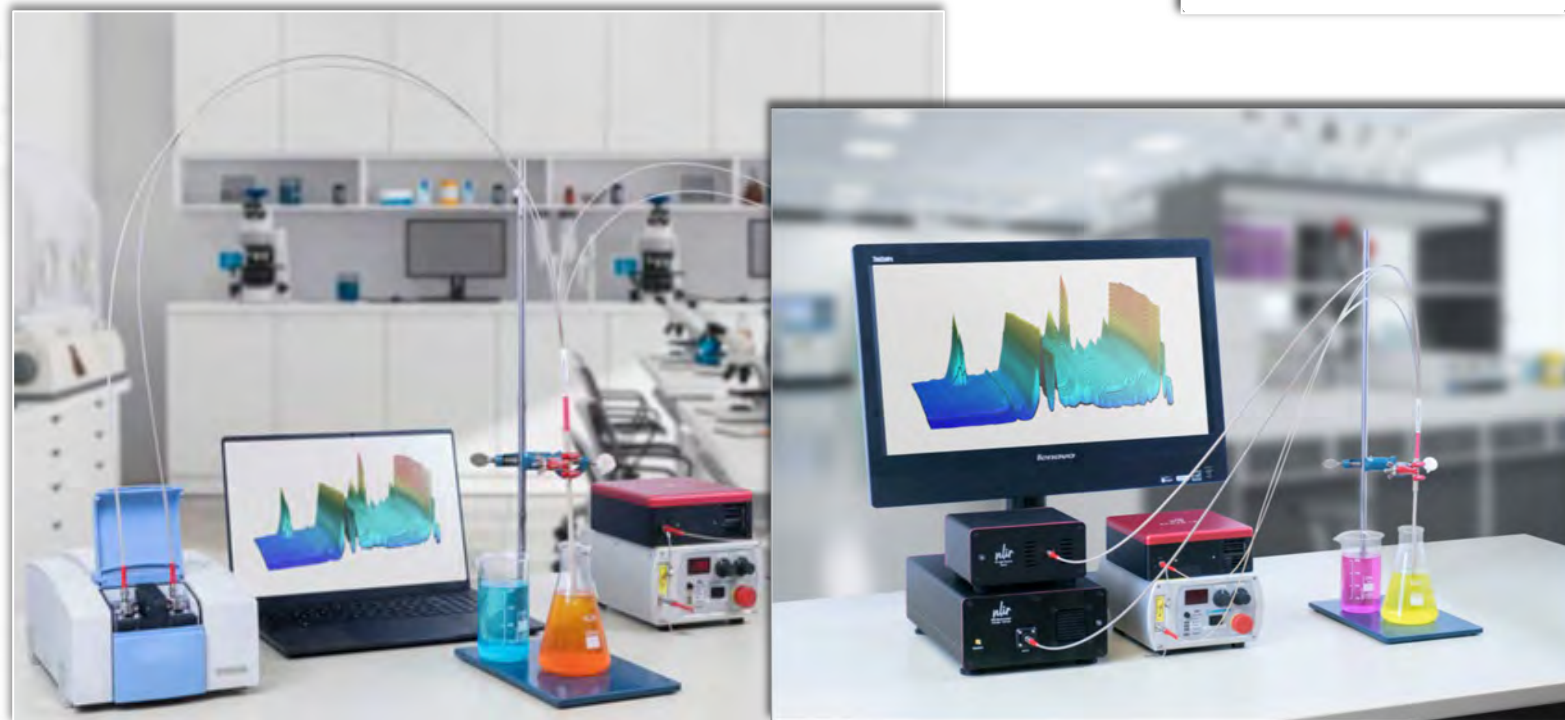
Combi-ATR/ Fluo&Raman Fiber System with Bruker ALPHA, NLIR & Wasatch spectrometers
