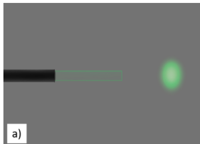
Bare Fiber with flat tip and conical flat emission profile (810nm to 980nm)
