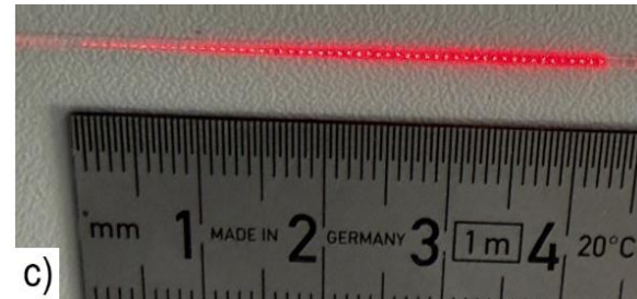
c) Transfer of the structures onto real silica fiber
