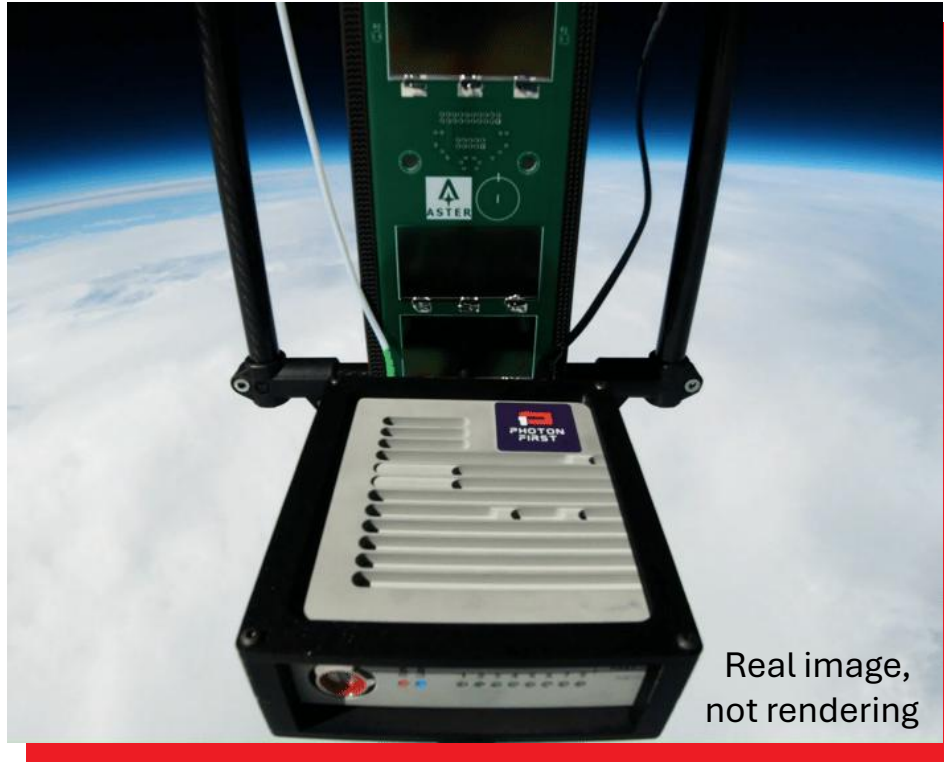
PhotonFirst's own FBG interrogator
