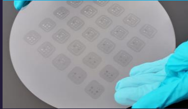
beam shaping optics mastering for NIL
