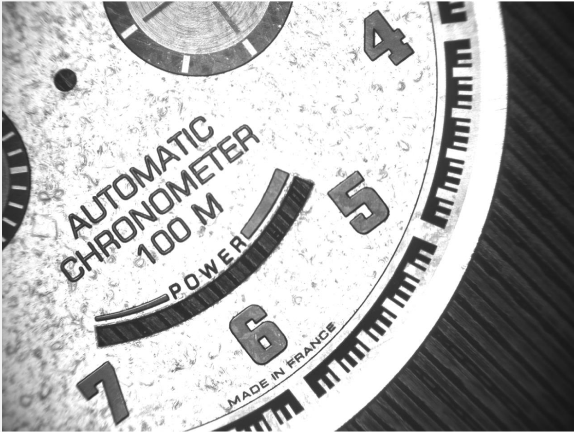
Picture 22x14mm with f.50mm : precision 20 \mu m
