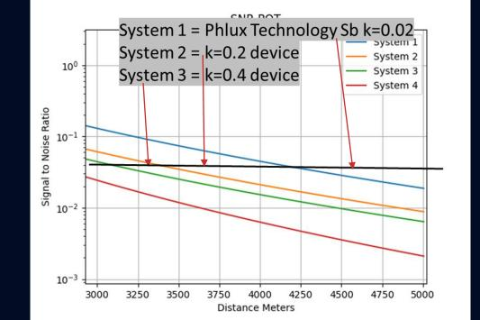
A Phlux Aura APD based LRF could have a Rx lens of 15mm diameter in comparison to a 25mm Rx lens for k=0.2 APD - yet still offer same performance. Or 20-30% longer range with same Rx optic – customer can choose which benefit he desires.
