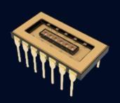
Ultra-High Gain - Operates like a SiPM but can detect at 1550 nm
