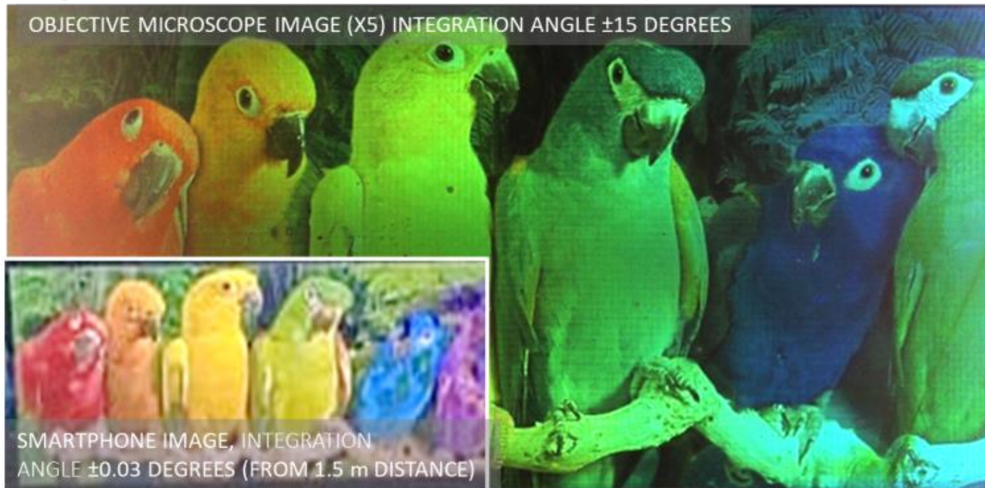
TiO 2 -based replica on glass
