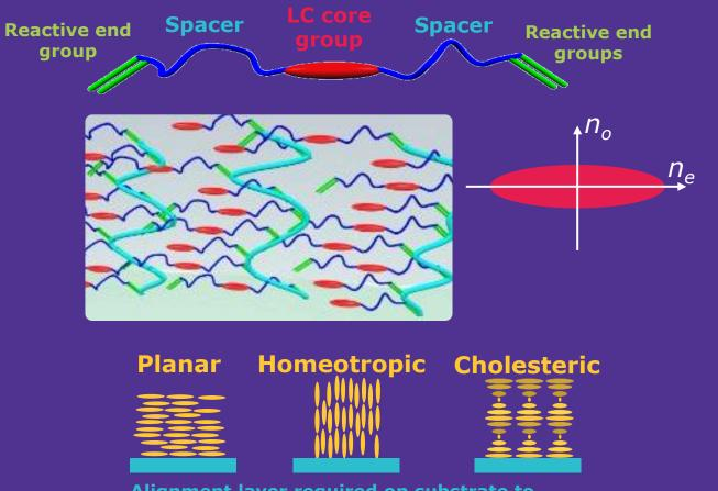
Alignment layer required on substrate to provide preferred direction to RM.
