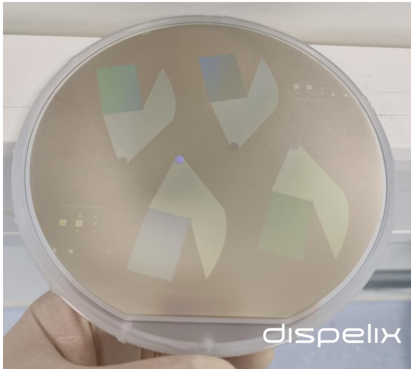
Augmented reality waveguides on 6in transparent substrate
