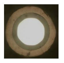
Octagonal fiber  $\phi$ core = 100 $\mu$ m NA = 0.2 Mode scrambling fiber designed for 1 $\mu$ m - 2.4 $\mu$ m
