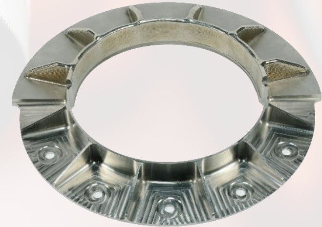
Heat treated and partially machined
