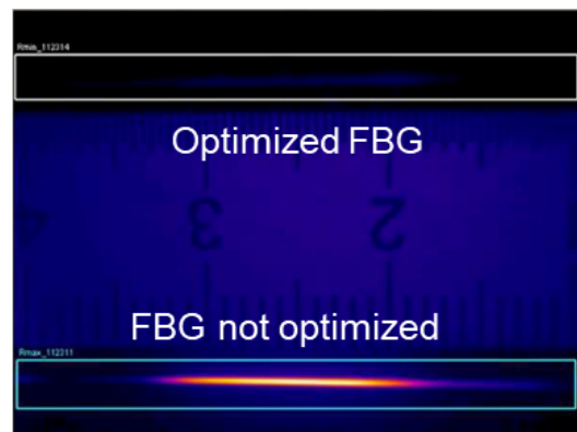
Thermal responses with IR thermograph
