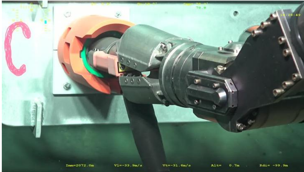
Connection to the Y junction box (using ROV Victor)
