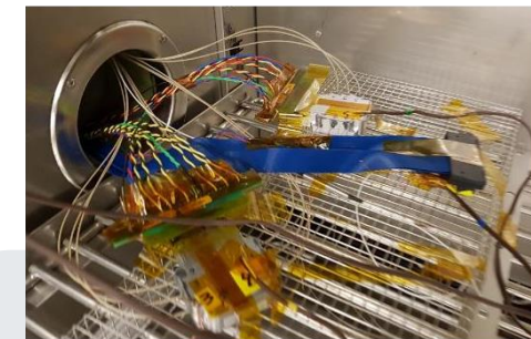
Damp heat climate chamber installation
