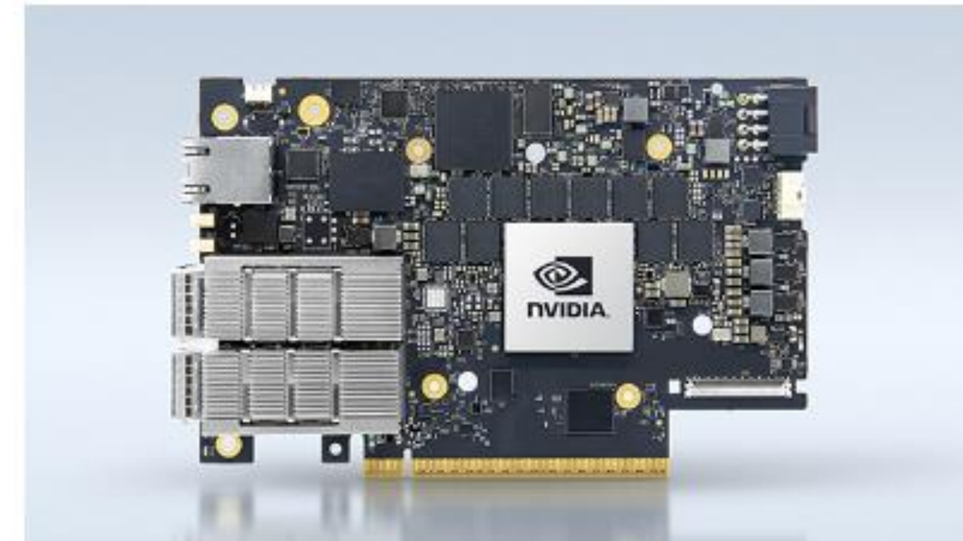
Data Process Unit (DPU)
