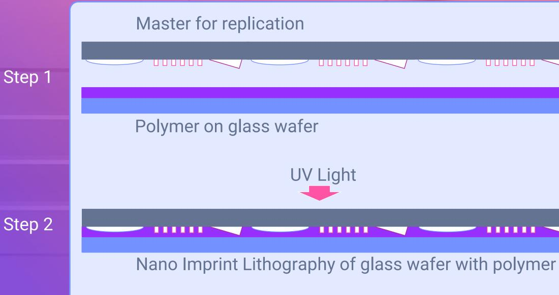
Wafer with NIL integrated optics ready for assembly
