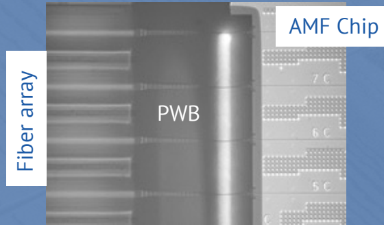
Loss per photonic wire bond: fiber to SOI Loopback
