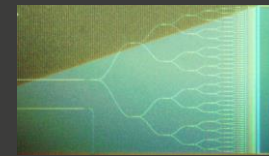
Si/SiO 2 grating couplers and waveguides - Interconnects
