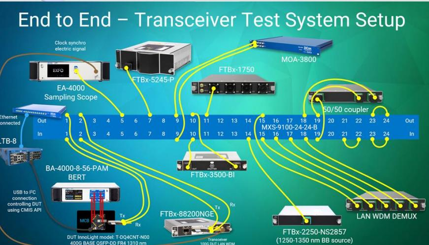
OptiInstrument communicates with instruments and automate their operation using remote control scripts
