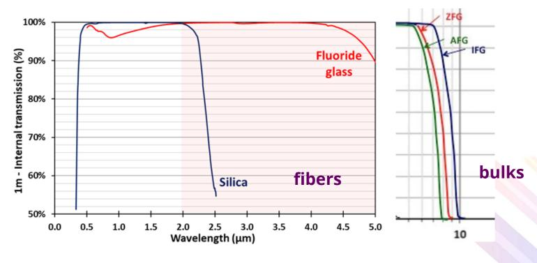
**Many rare-earth transitions** for lasers and amplifiers in the visible, the near infrared and the midinfrared (dopants: Dy, Er, Ho, Nd, Pr, Sm, Tm, Yb,... numerous codopings, at concentration up to 10 mol. %)
