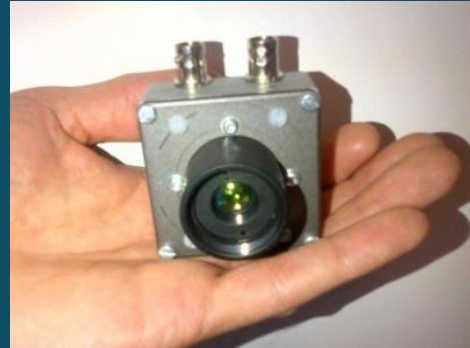
Modulated retro-reflector based on MQW technology provided by RISE (Acreo)
