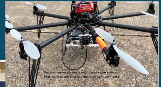
Modulated retro-reflector based on MQW technology provided by RISE (Acreo)
