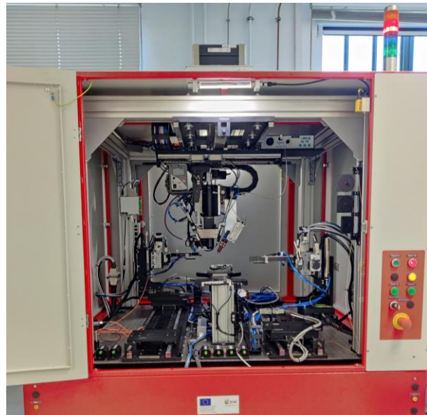
Automatic alignment and standard attachment of fibers
