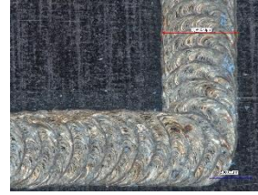
Busbar welding on battery module
