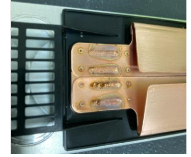
MODULE/ PACK ASSEMBLY WELDING
