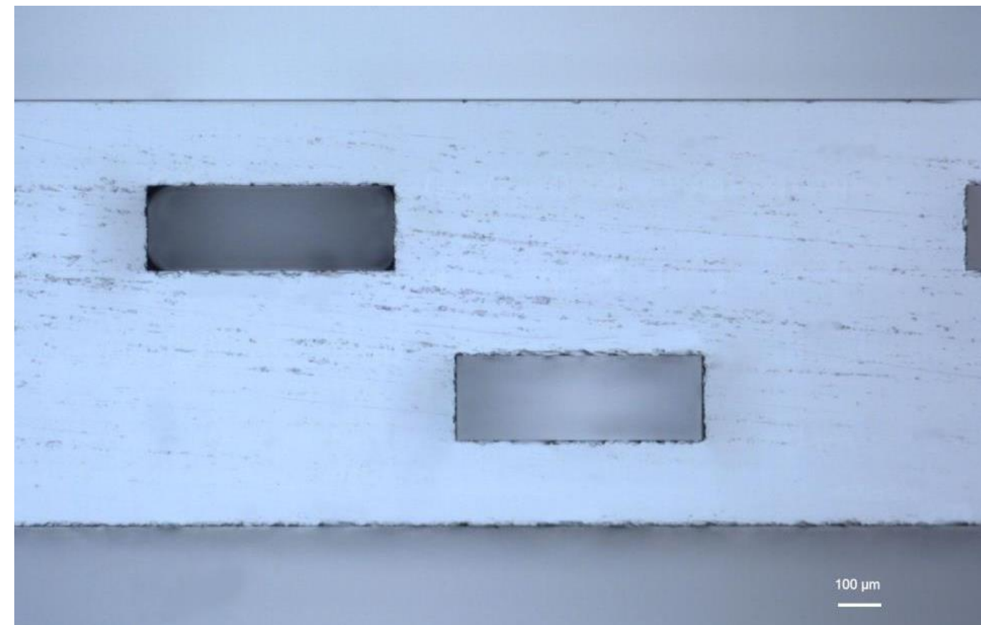
Microfluidic chip, 5 hermetic layers bonded without adhesive, side view
