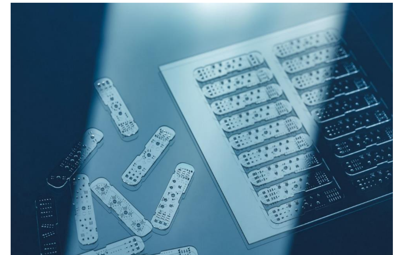
Switch ceramics to glass for probe cards to reach 80% less defects and 20x faster processing
