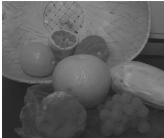
At 940 nm NIR image sensor shows no major contrast. Mold in grapes not visible at all
