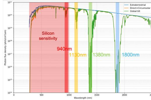
Can image in **solar blind regions** removing sun ambient noise and glare for **better sensitivity/SNR**
