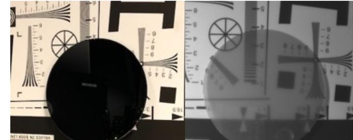
**Silicon is transparent to SWIR light** enabling SWIR imaging through Si based devices
