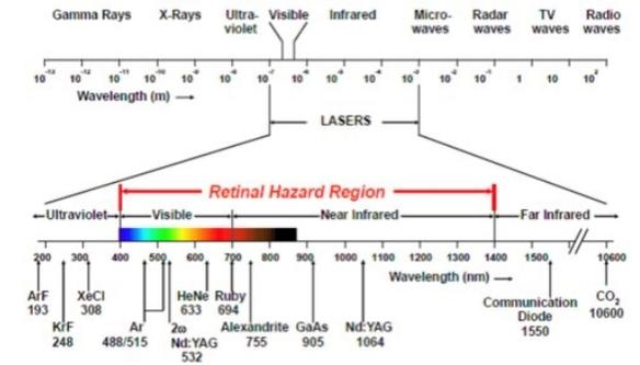
>10X safer for the eye providing higher brightness illumination and **better SNR**
