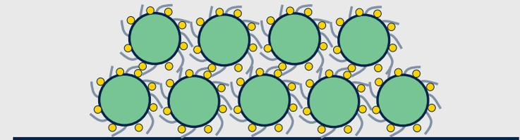
Proprietary processing enables the creation of highly dense QD films with improved charge transport and passivated trap states
