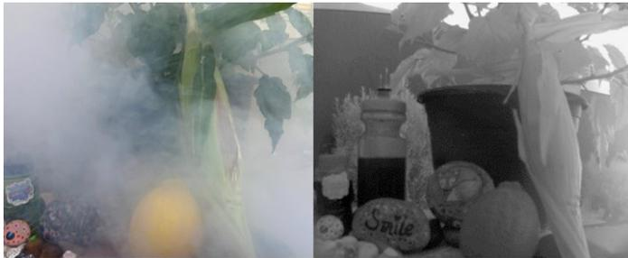
SWIR light is scattered less by particles suspended in air (**higher penetration coefficient**) making it possible to **see through fog, smoke, rain, snow**, etc.
