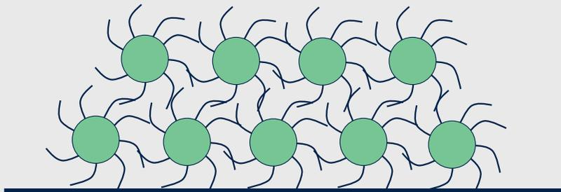
Colloidal QDs dispersed in solution are dispensed on wafer by spin-coating
