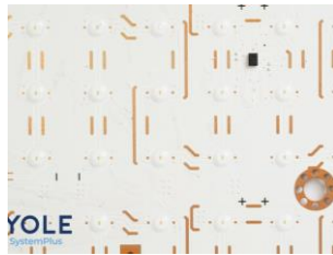
Mini-LED backlight unit in Odyssey Neo G9 49" Samsung Monitor
