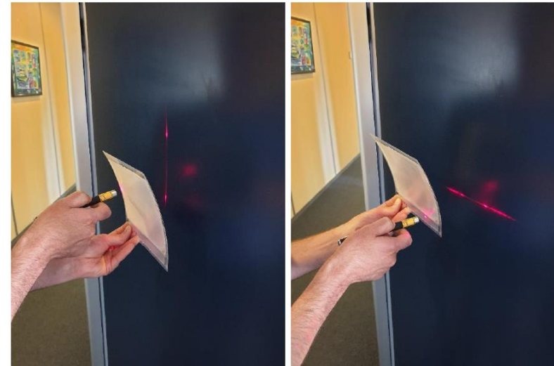
Effect of one direction prism imprint on laser light.
