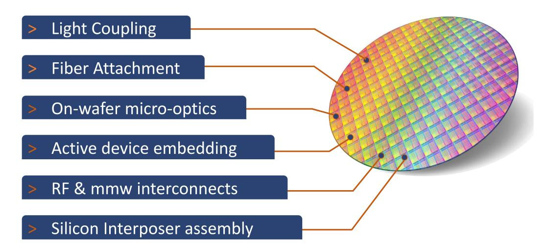
Combination of functionalities using scalable Waferlevel Microfabrication techniques
