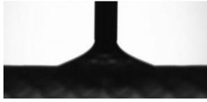
Deposition of hydrophilic solutions on hydrophobic / super-hydrophobic surfaces will impact resolution
