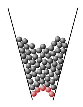
Particle size < 10% of tip diameter to avoid jamming
