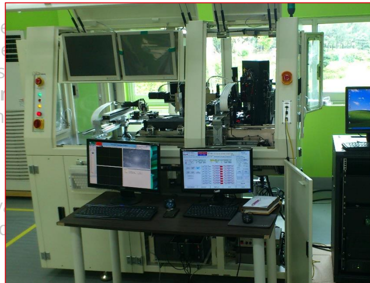
Automated test bench for focus measurement
