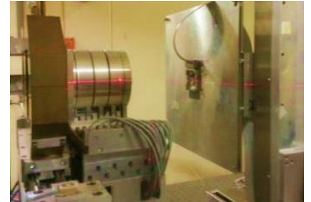
Proton radiation tests on PIC Interrogator modules
