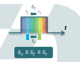
This phase change is equivalent to a frequency drift inside the chirped pulse.
