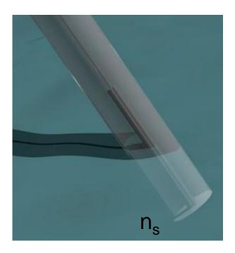
The amplitude of the interference pattern changes with n<sub>s</sub>.
