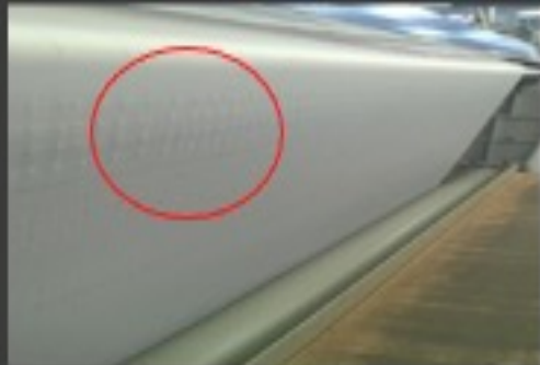
Fiber Optics Woven in Test Fabric
