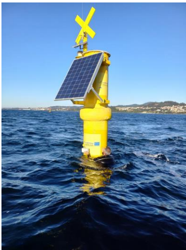
Multimaterial off-shore wind tower scale (1:10) with embedded metallic coated FOS to monitor corrosion
