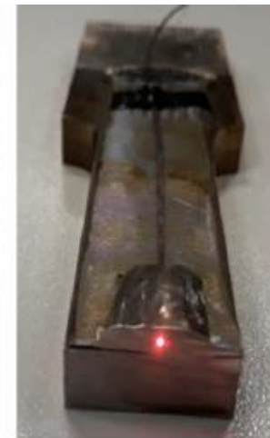
Embedded Ni coated FOS in the antifriction material by manual and laser TIG welding
