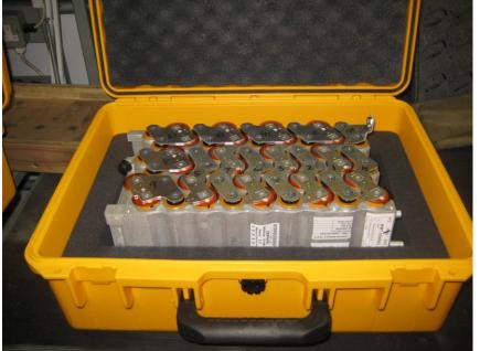
Examples of laser welds in module interconnects.
