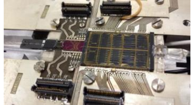
Photonics-based beamforming antenna system for broadband satellite communication, LioniX International.
