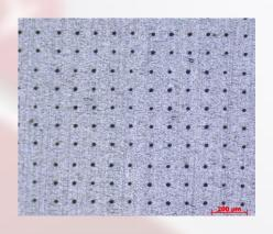
12500 holes/s in SS with 12,5W 20µm diameter holes 92% roundness
