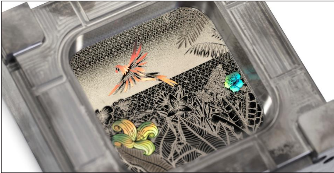
Femtosecond laser micro-milling over tempered steel mold
