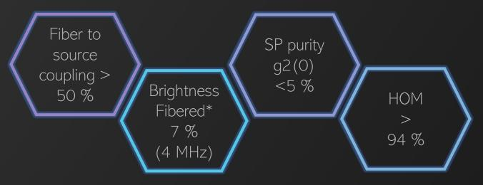
\* Brightness fibered for standard active alignment = 25 %
