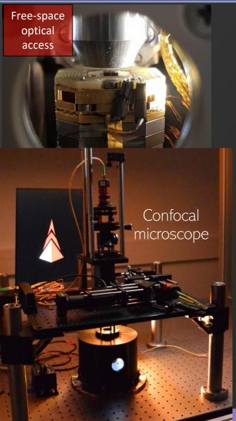
Based on a low-vibration cryostat with active alignment (nanopositioners)
