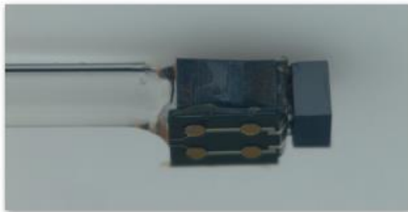
Fiber aligned to VCSEL and bonded
