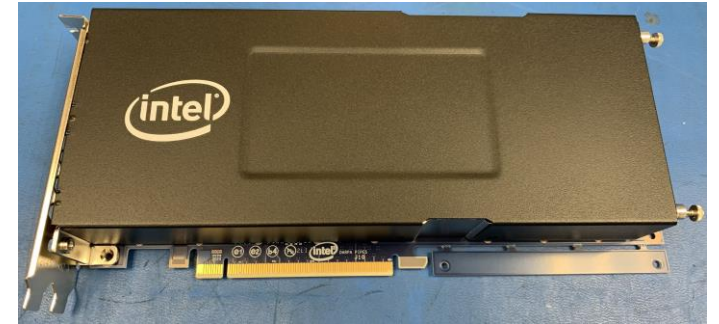
Intel® FPGA Optical Programmable Accelerator Card (O-PAC) Prototype • PCI-E Form Factor
