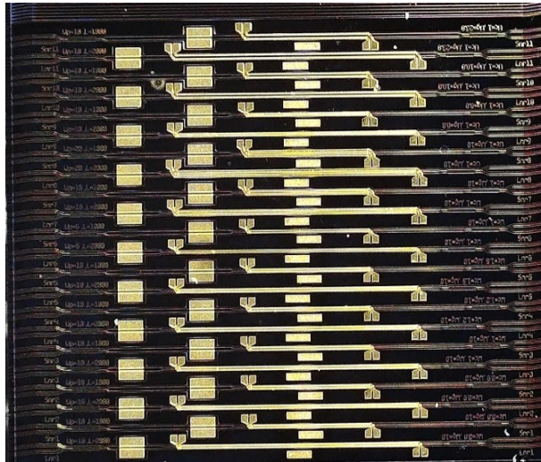
High density Mach-Zehnder modulators on a 4.6 x 4.0 mm 2 MPW cell
