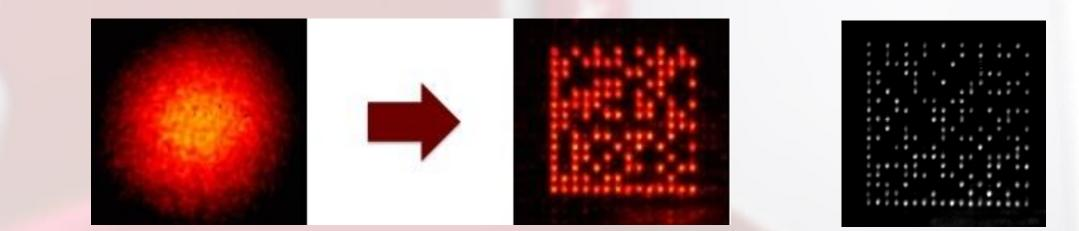
VULQ1 patented Multibeam technology allows to generate 10, 100 or 1000 laser beamlets on-demand, from one single laser beam.
