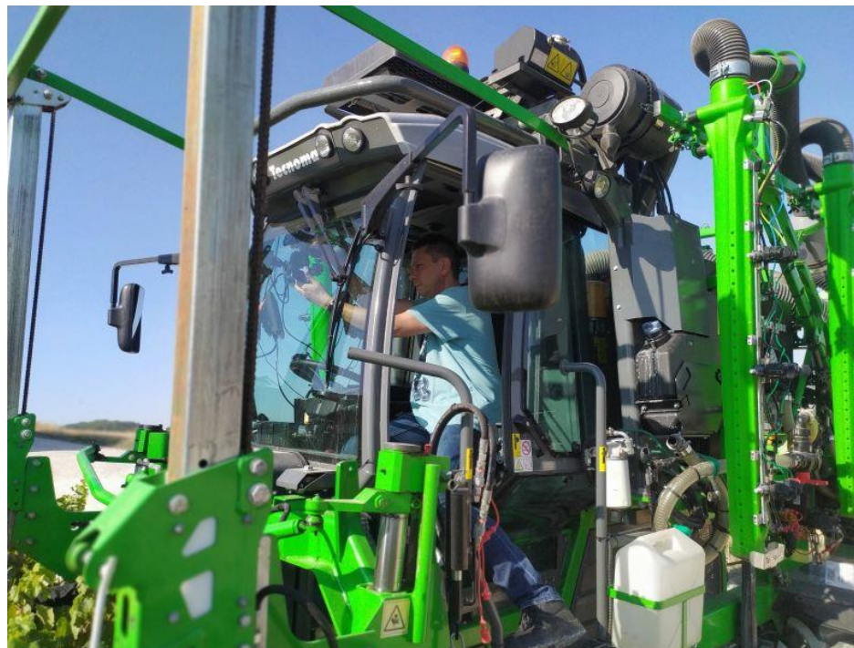
Positioning the TOUCAN camera (in a dedicated body) onto a vineyard straddle tractor.
