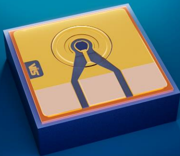
InP Photo-Diodes for 112 Gbit/s PAM-4 >0.5 A/W from 850 nm to 1550 nm
