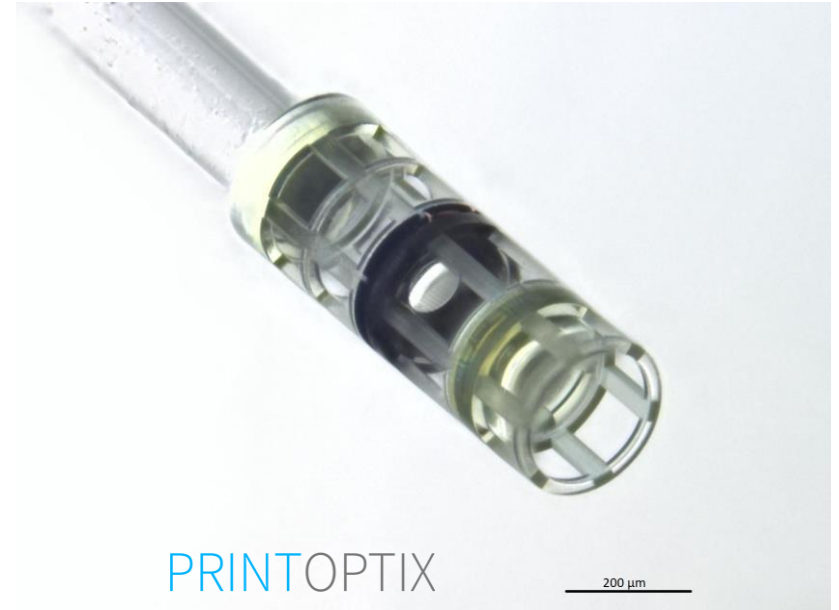
Imaging system with central aperture on the tip of a 160 \mu\text{m} imaging fiber.
