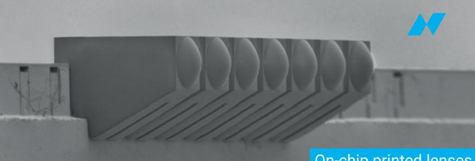
On-chip printed lenses for free space microoptical coupling
