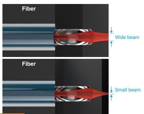
Beam expander for relaxed alignment tolerances in packaging
