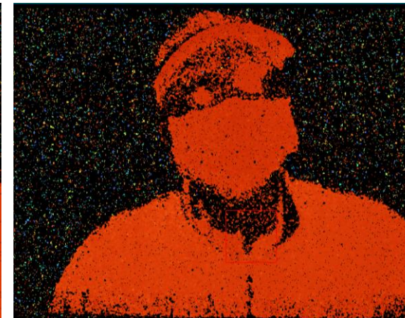
Outdoor scene captured with 1380nm proof-of- concept 3D Depth camera - the sun is gone!
